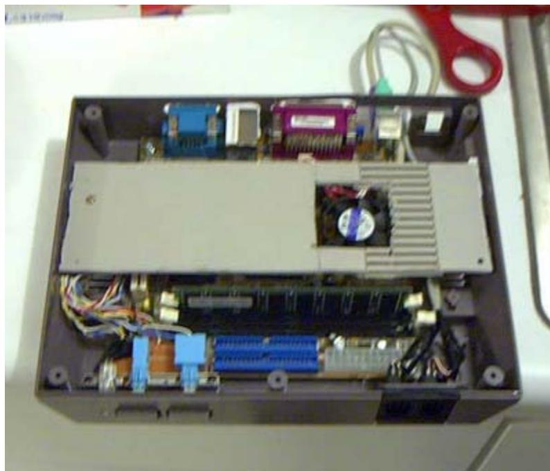
I laid the motherboard in where it belonged, and measured how large my shelf should be. It's 3 inches by 7 inches. The screw holding it in on the left side screws into the regular nub that we left while gutting the case. The right side is held on by 2 L brackets that are hidden in the indent
