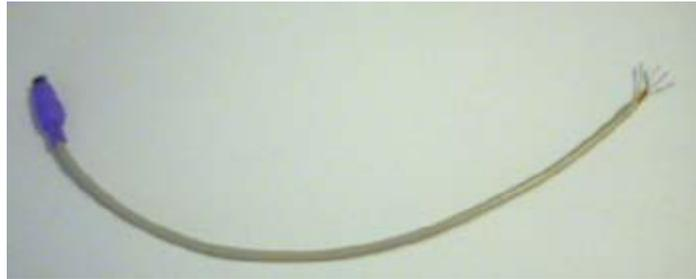
I cut off a small section of the regular keyboard wire and stripped the wires inside.
