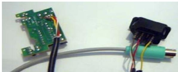
With my mouse, the Nintendo controller wires had to be soldered directly onto the circuit board inside my mouse. However, the basic principles remained the same. I just had to make sure the wire in my board was connected to the wire that connected to the right wire in my mouse plug. I know it sounds confusing, but it's not that bad, really.
