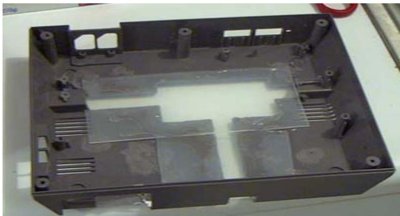
Because you don't want the bottom of the motherboard sticking out of the computer, it's important to line the bottom of the Nintendo with something to keep it off the ground. Any thin plastic will do. I used clear plastic, because I thought it looked cool. It's being held down with some epoxy, but any glue will do.
