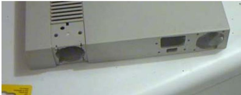
You'll need a place to plug in your power. It's also extremely important to keep the air in the case circulating. The power supply will get very hot, and it's mounted very close to the processor. You have to keep the air moving out, or you will have heating problems. Above is an image of what the top of my case looked like after cutting all the holes. The fans I bought at a local computer shop for \$3.00 each. The one on the left blends in perfectly with the black stripe along the top.
