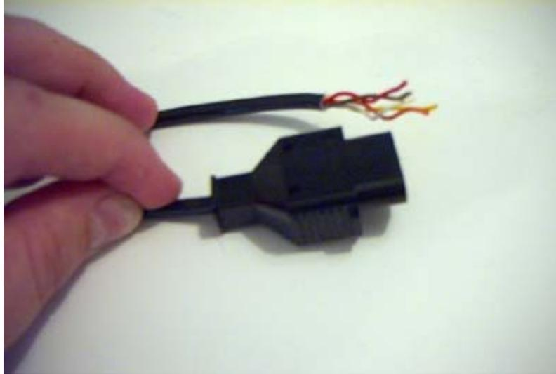
Here's the cut end of the Nintendo controller. The wires are shown above. While stripping these wires, you may get a bit frightened. They're not exactly wires you see every day. They're tightly wound strips of metal. While stripping, you'll probably unwind this metal and make it very thin. I recommend using an X-Acto knife to cut away the cover rather than regular wire cutters for this reason. However, you solder these wires exactly the way you solder regular wires.
