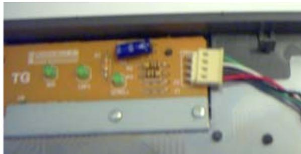
This is what makes my keyboard work. I had to cut the cable at this point and put in the Nintendo cable instead. If I were you, I would write down colors so you don't forget. For example...
