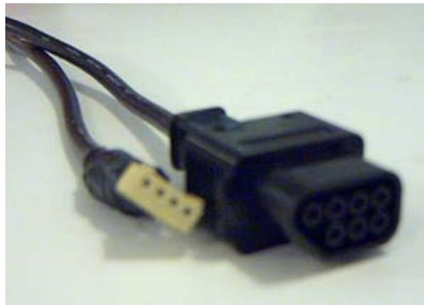
Here I soldered on the Nintendo wires to the keyboard wires in the picture above, making sure to remember which color wire connected to which.
