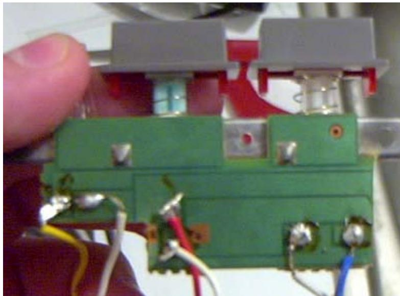
Here I soldered on all the wires to make it work. On the left are the 2 wires for the LED light. In the middle, the power switch. On the right, the reset button. I also coated the back of the switches with electrical tape at this point. It was so close to the motherboard that I didn't trust it unprotected. The electrical tape stops any electrical interference that may happen, because it is non-conductive.
