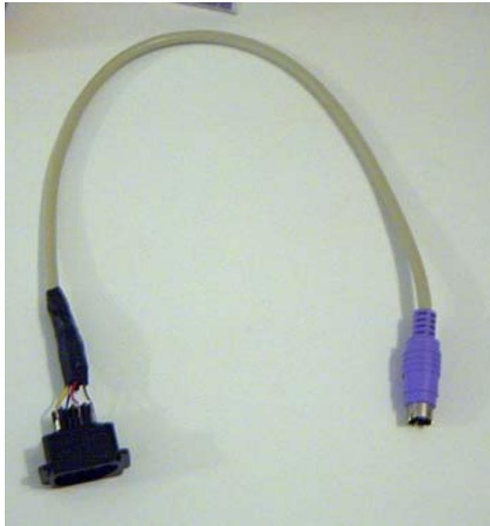
Now, I connected the keyboard wire to the Nintendo plug. So keyboard red went to Nintendo brown which went to keyboard red. All the connections remained the same, but you just inserted different wires in the middle. I know it's a bit confusing at first, but if you really want to make this work, it's not that hard to figure out. The mouse needed to be modified the same way, with 1 little exception.
